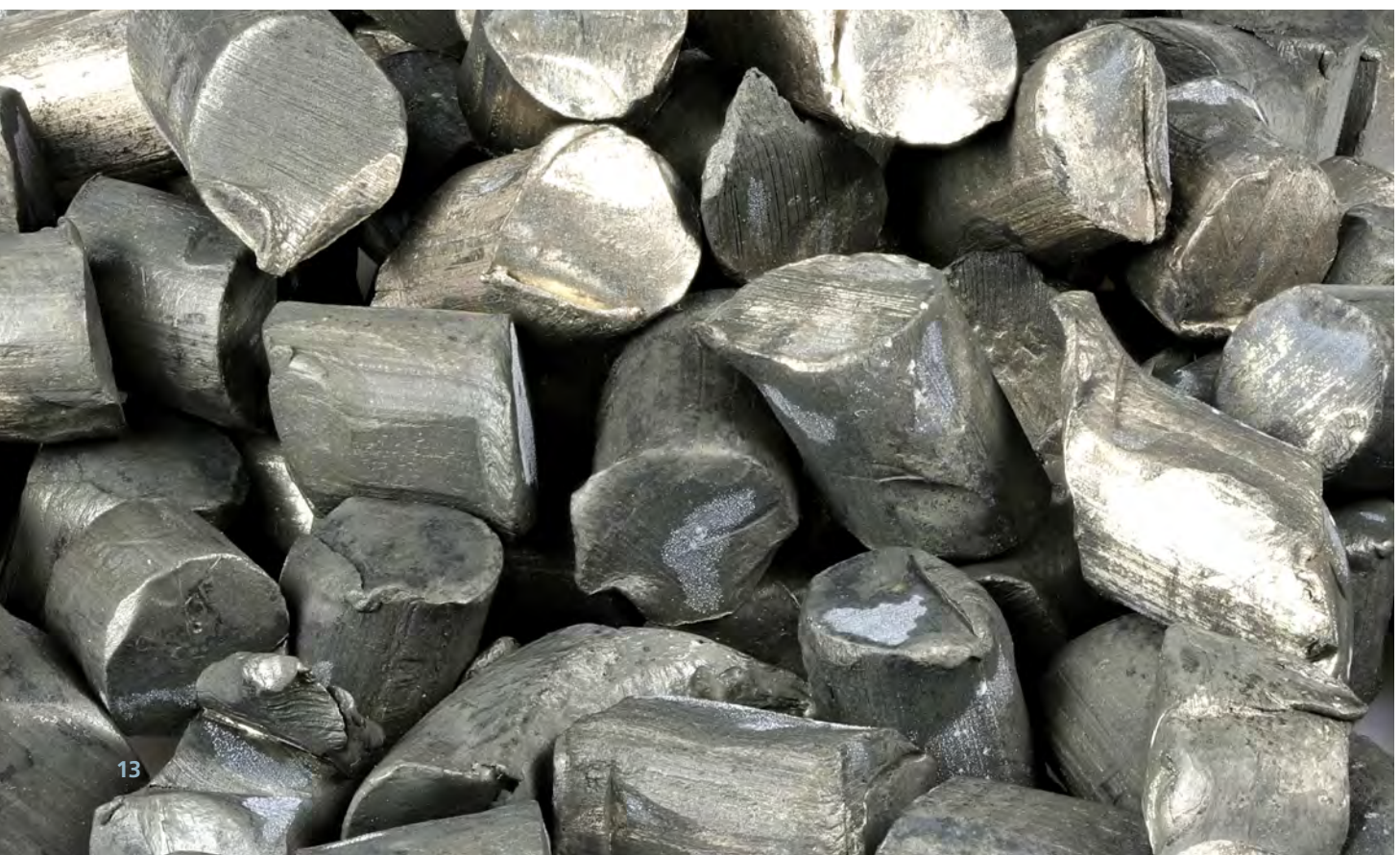
Lithium granules as feedstock for evaporation
