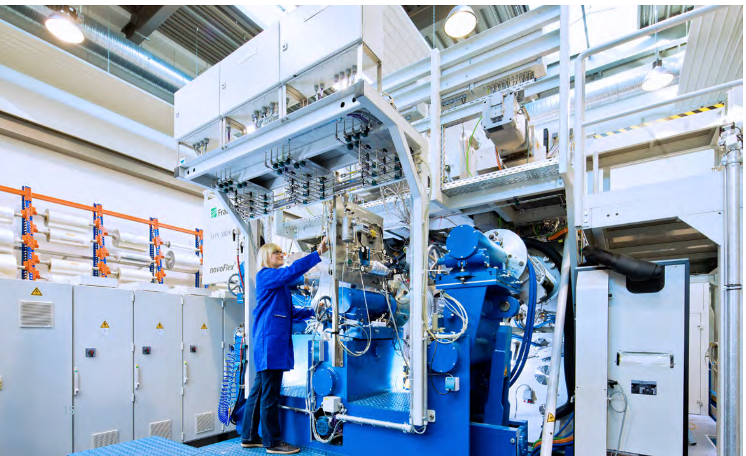
navoFlex® 600 – Roll-to-roll pilot web coater
